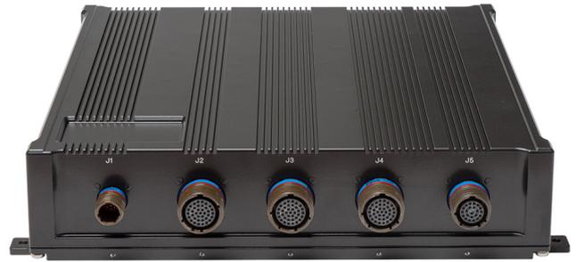
The MIL-PIP46-C12 comes with interfaces like 3x DVI-D, 4x USB 2.0, Audio, dual LAN, and a wide power input. Additional expansions can be done over the internal expansion interfaces such as mPCIe, m.2, or PCIe/104, These expansions can be done easy and quickly be integrated into the system. This makes the solution flexible and cost efficient customizable.
