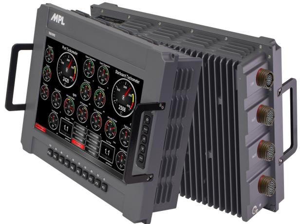
The system is designed with a military grade, high strength, and light weight housing (SWaP-C). The enclosure meets IP54 all around. Its modular architecture allows the system to be easily configurable with many options (GPS, 1553, WLAN, LTE...). Additional function keys for faster operation of the system can be implemented. An expansion with GPU for compute-intensive applications such as image processing, can easily be integrated.
