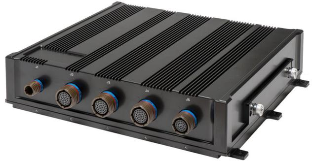
The PIP Family used in mission control computers and servers, is explicitly designed to withstand extreme environment conditions. It starts with the design of the CPU board, the adapter board to reduce/eliminate cable connections as much as possible, and ends with the selection of the parts. The design experience and success since 1985, allows MPL AG to design the most rugged and reliable solutions, customers have been depending on for decades.
