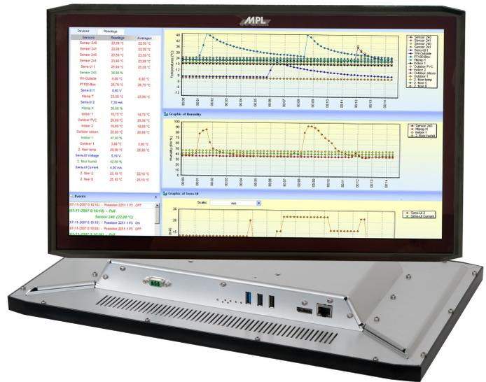
The front of the PANEL18 is an IP65 protected, powder coated aluminum frame. On the back are standard interfaces available (can be customized). The Solution can be equipped with M12 to be used in Railways or Maritime application, other connectors are available on request. The standard supply power is 12VDC or optionally with 9-36VDC / 48VDC or 110VDC. Like all other MPL products, the PANEL18 does not require a fan, is very flexible, and can be adjusted to the customer needs and requirements.
