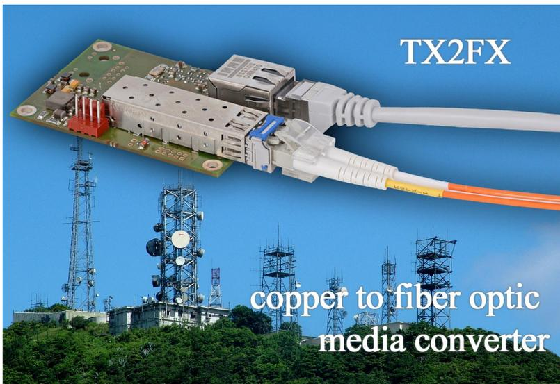
For the optical port the TX2FX supports Small Form-factor Pluggable (SFP) transceivers. SFPs enable adaptability to different fiber types, distances and wavelengths, providing maximum flexibility across a variety of network architectures and topologies. SFP ports are ideal for flexible choices of the transceiver distance needed.
