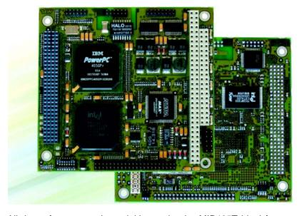
The MIP405T is intended and designed for use in hardest environments with operating temperature ranging from -40°C to +85°C without the need of a heat sink or a fan. Special efforts have been taken on the quality of the components and their long term availability as well as on the low power consumption of the system which is less than 3 Watts at 400MHz.
