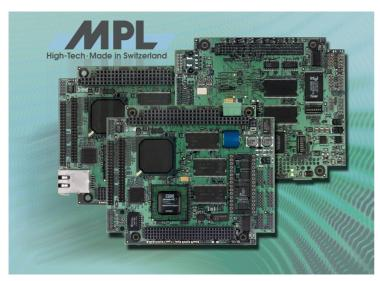
The MIP405 can be used in environments of up to – 40°C to +85°C without the need of a heat sink or a fan. Special efforts have been taken on the quality of the components and their long term availability as well as the low power consumption of the system which is less than 3 Watts at 400MHz.
